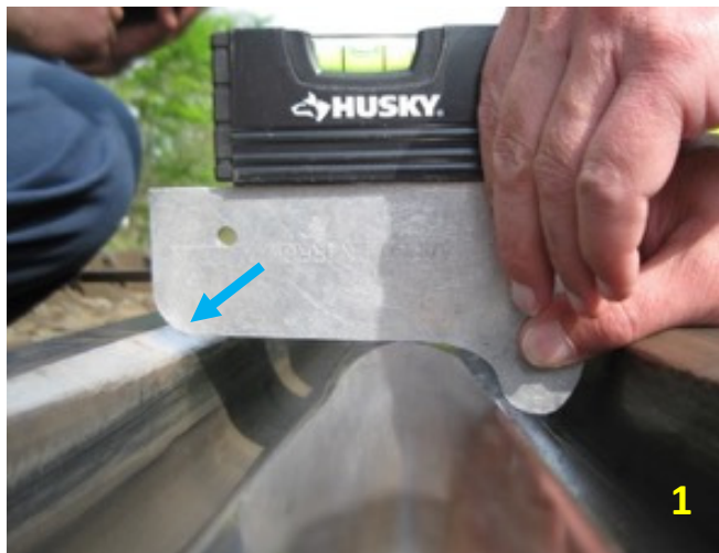
A new wheel has full bearing on point, with clearance between wheel and wing.
