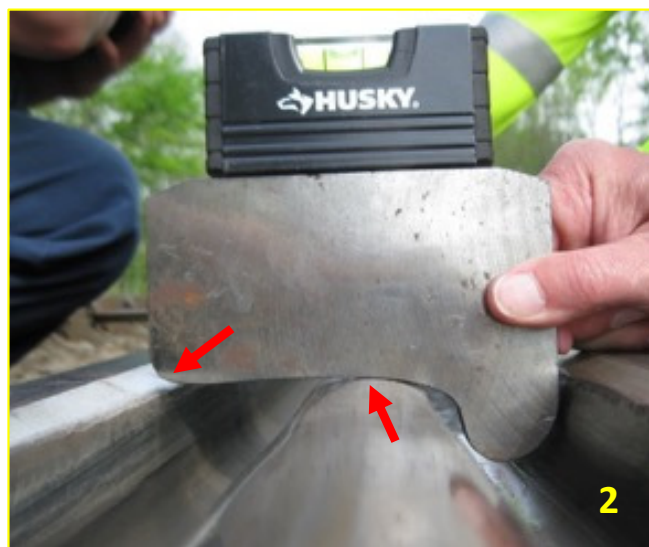
A 1-mm hollow wheel is riding on both the point and the wing.
