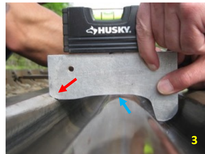
A 1-mm hollow wheel is riding on both the point and the wing.
